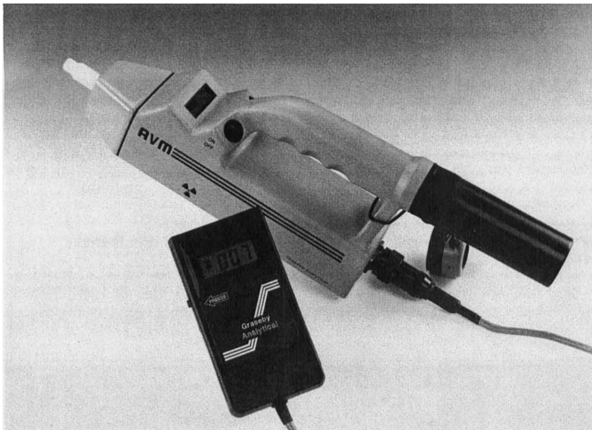
FIGURE 12. The ion mobility spectrometer with digital display unit manufactured by Graseby Analytical, Ltd. Used with permission.
